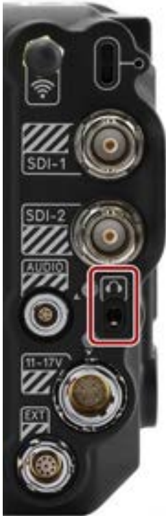
Figure: Front face of the female 3.5 mm headphone jack (looking at the back of the camera).
