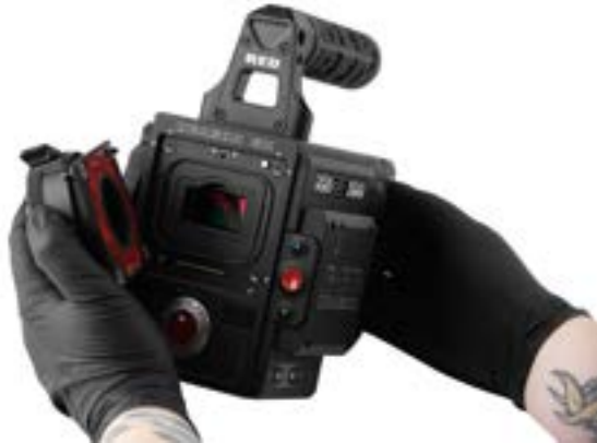
Figure: Remove the Lens Mount
