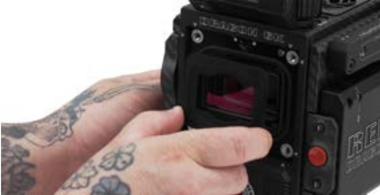
Figure: Remove the OLPF Module
