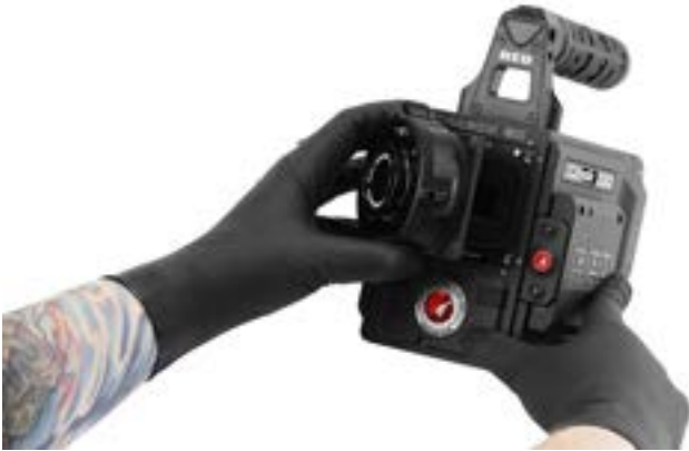
Figure: Align Lens Mount Pins
