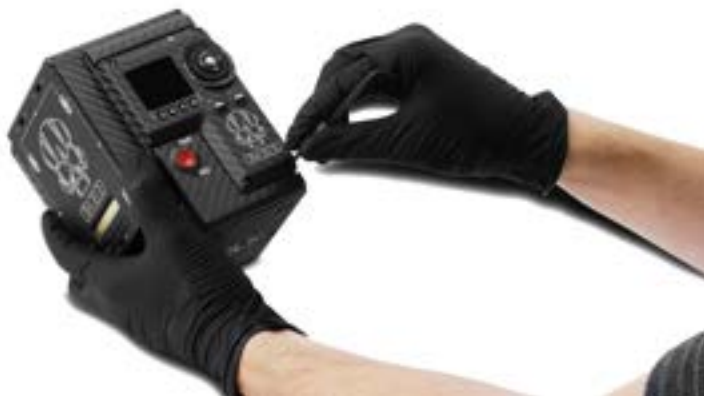
Figure: Reinstall the Side Module/Panel
