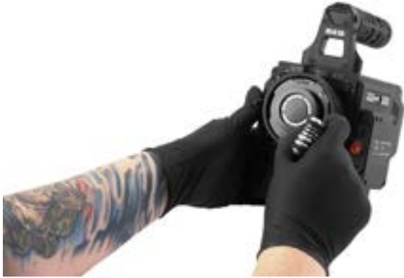
Figure: Remove the Lens Mount Screws
