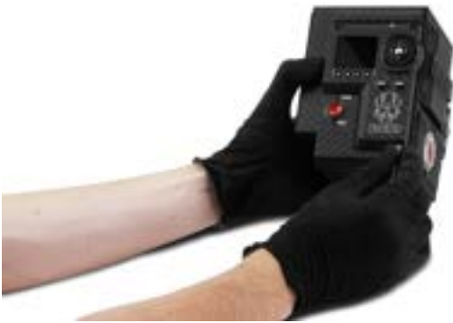
Figure: Remove the Side Module/Panel
