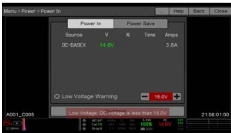
Figure: Low Voltage Warning
