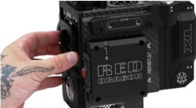
Figure: Install the New OLPF Module
