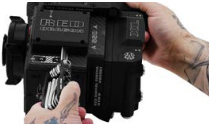
Figure: Remove the Focus Hook Screw
