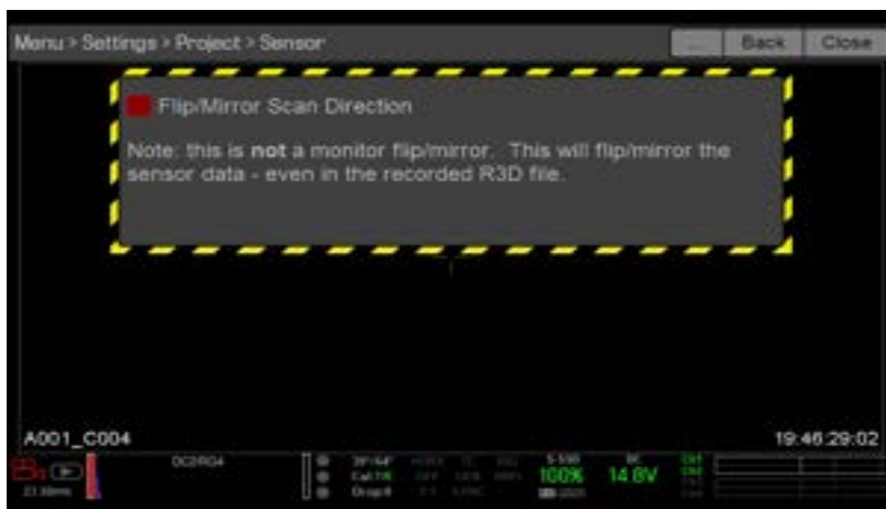
Figure: Flip/Mirror Scan Direction
