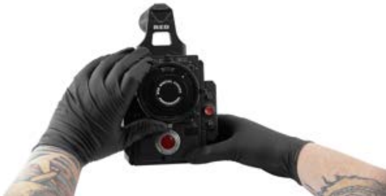
Figure: Turn Locking Ring Counter-Clockwise
