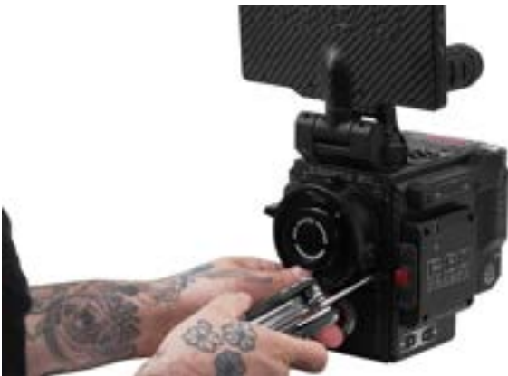
Figure: Remove the OLPF Module
