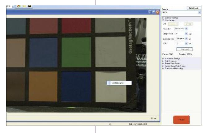
Beneath the Camera selector are a series of expandable headers which contain groups of related camera settings.
