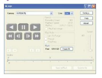
Scrub through a clip by dragging the play head back and forth on the timeline. Use the playback controls to play forward and in reverse. Use the speed slider to change the playback speed.
