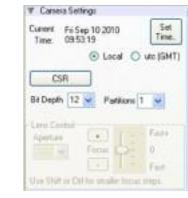
From the Camera Settings section you can set the time of the internal clock in the camera. This will affect the time stamps that are embedded in the recorded cines. The simplest way to set the time is to click the "SetTime..." button, then in the resultant pop-up window click the "Update and Set" button. This will set the camera's time to the computer's time.
