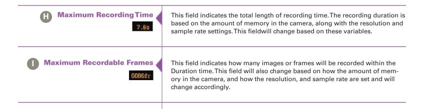
Menu for Setup and Recording Parameters
