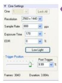
The most common shooting parameters are set in the "Cine Settings" section. Resolution, Sample Rate (i.e. frame rate) and Exposure Time (i.e. shutter) can be set by choosing a setting from the appropriate pull-down menu. If you wish to use a setting that doesn't appear in the menu, type in the value you with to use. If you type in a value that isn't supported by the camera, the software will round the value to the closest supported value.
